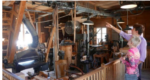
The belt driven equipment at the furniture factory
